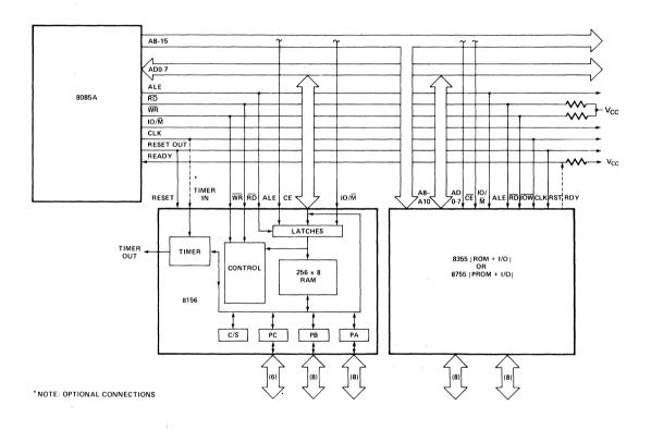
Figure 11. 8085A Minimum System Configuration. (Memory Mapped I/O)
